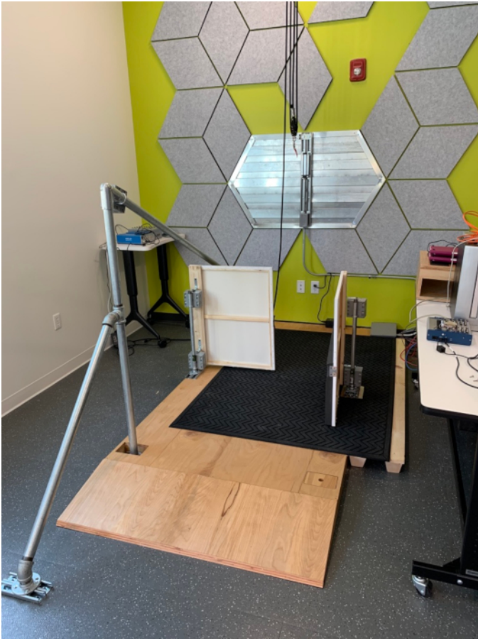
Figure 1. Lean & release setup with leg blocks. In this example, one leg block is set in the open position, while the other is set to prevent a step. These blocks are moved via computer-controlled motors (grey boxes attached to the support posts). Handle covers are also moved to either block or allow a reach-to-grasp response. Here, the covers are detached to allow full view of the handle. The release magnet is visible on the back wall. All the wiring feeds through the wooden platform itself and enters into the grey circuit box located on the back corner. Please click here to view a larger version of this figure.
