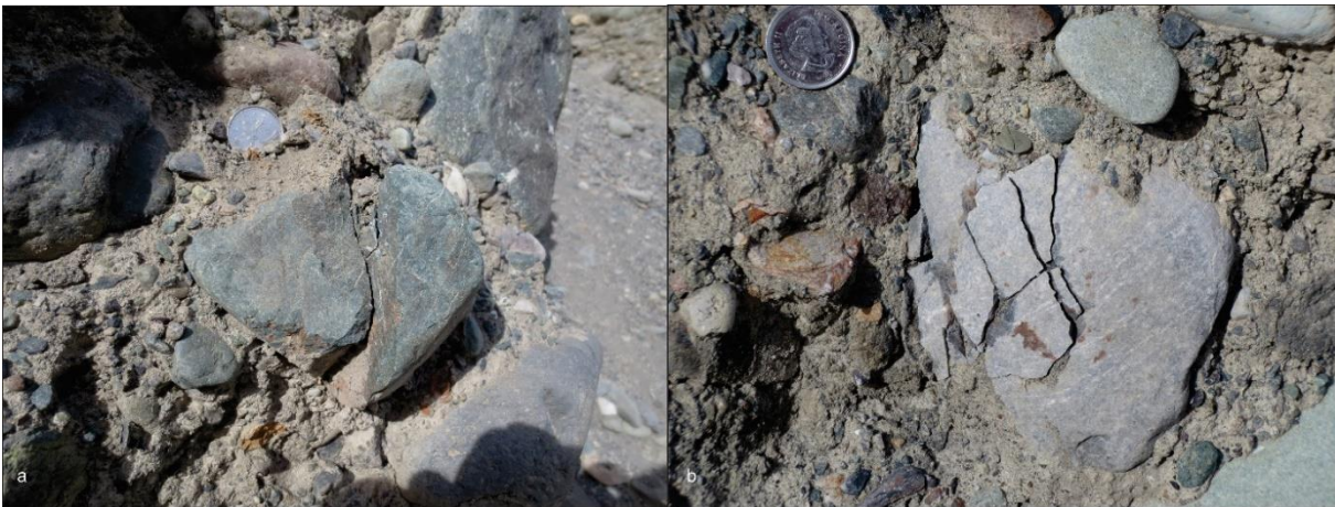
Figures 10. Fractured pebbles and cobbles within the Denali fault zone in the Duke River bluff
