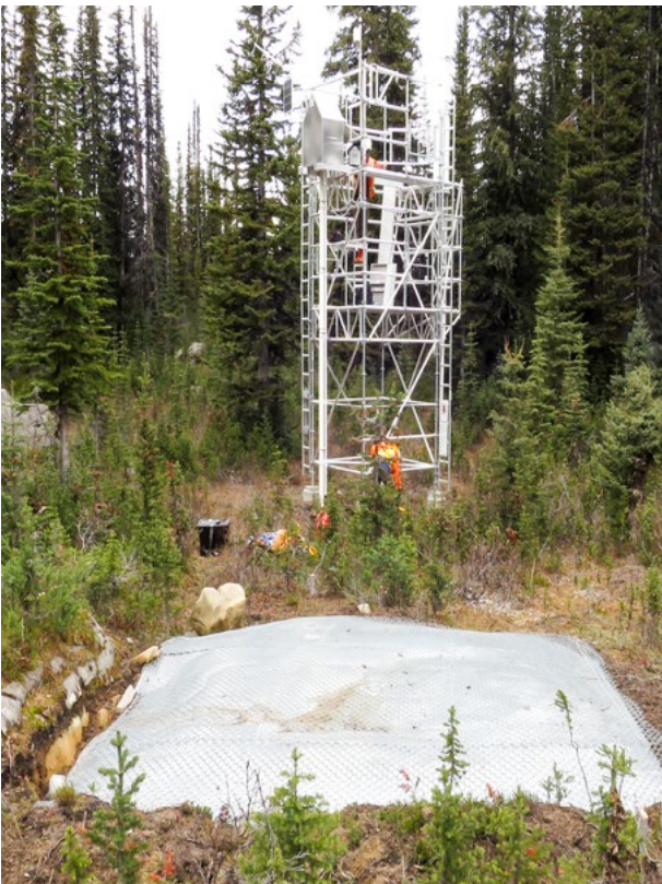
Figure 3.13 Custom-built snow pillow with open hydraulic system and shaft encoder.
