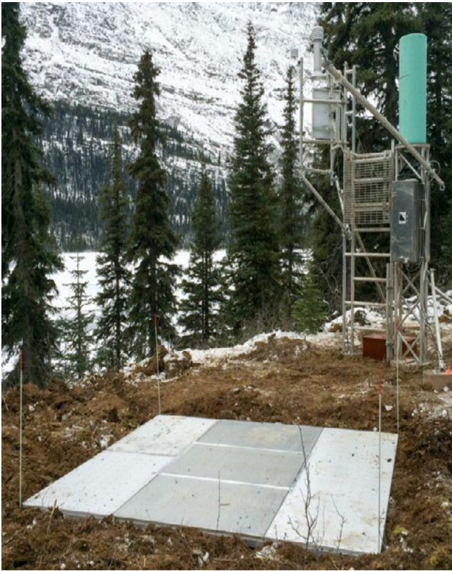
Figure 3.15 Sommer GmbH SSG1 snow scale.
