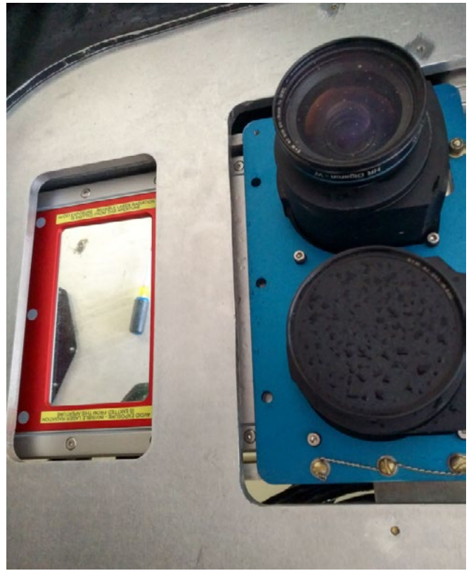
Figure 3.16 Lidar sensor (on the left) mounted at the floor of the aircraft.
