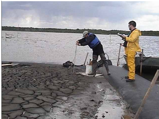
Figure 12. Engineers are shown standing on a tube taking samples on May 22. The sediment developed dessication cracks almost immediately and consolidated rapidly. Despite high water, which flooded the island during most of June, researchers could walk on it in early July.
