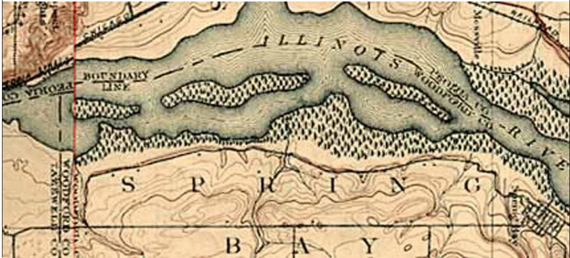
Figure 1. This topographic map from about 1890 shows Upper Peoria Lake between the narrows and Spring Bay (lower right). The Stippled area is marsh and three islands are clearly visible. The islands, marsh and some floodplain were covered with water by the navigation dam. Sediment removed to deepen the lake could be placed on the old islands restoring both aquatic and island habitat.
