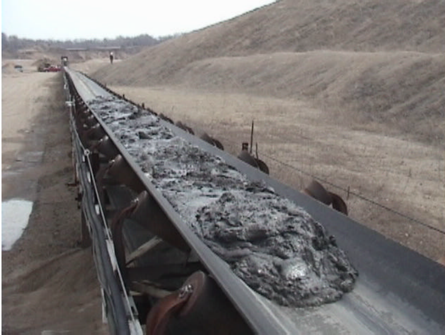
Figure 9. Peoria Lake sediment after a 600 foot run on a 36 inch conveyor belt. The material was excavated with a clamshell, barged to the site, clam shelled into an end loader bucket and placed on the belt within three hours of excavation. The sediment maintained its cross section during the run.
