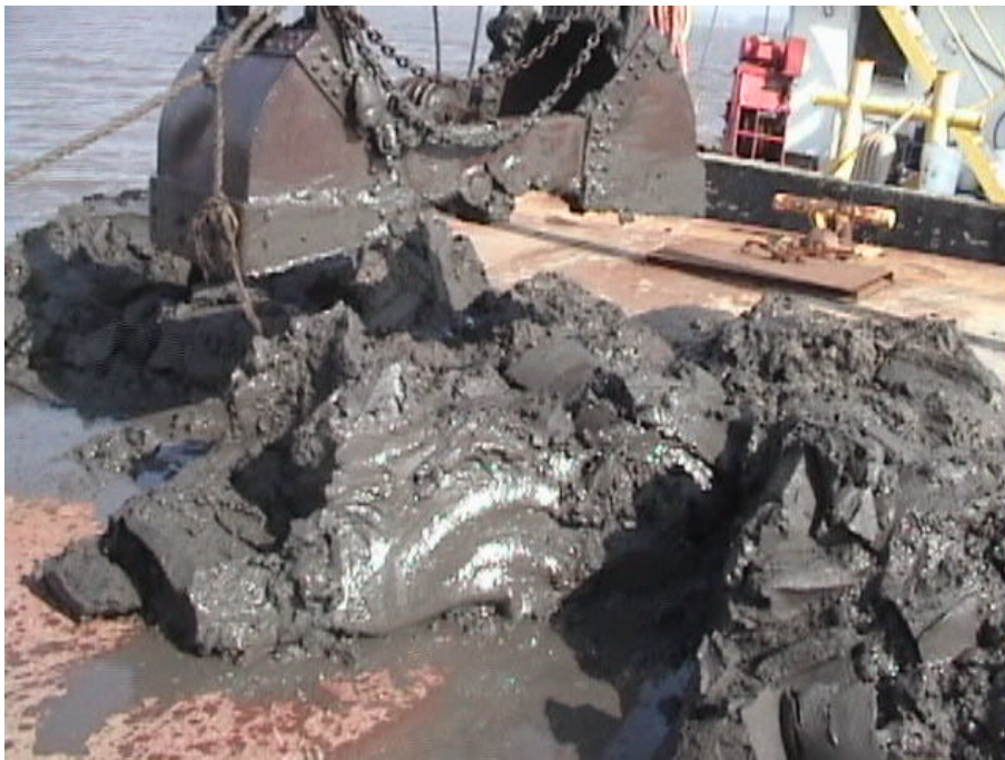
Figure 6. Sediment deposited in Upper Peoria Lake since 1900 is generally stiff and has the consistency of cookie dough. The sediment in this picture was used in the conveyor demonstration within three hours of excavation.
