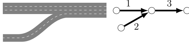
Figure 7.4: Sketch of a merging junction consisting of three links.
