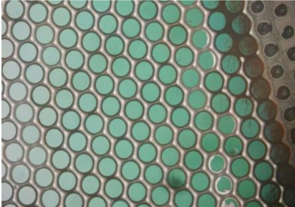
Figure 6.16 – 150 \mu\text{m} diameter pin-fin heads after fracture (covered by glass and dye)
