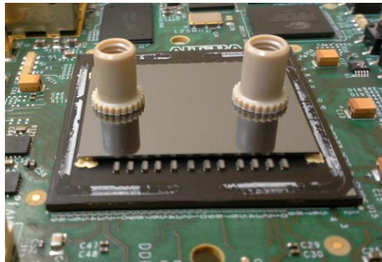
Figure 2.16 – FPGA device with embedded microfluidic cooling system mounted on board. Image originally shown by [11].
