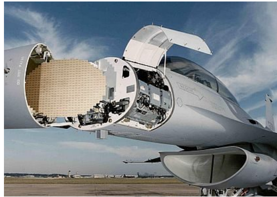
Figure 1.2: An example of a passive phased array system embedded into a plane. [7]
