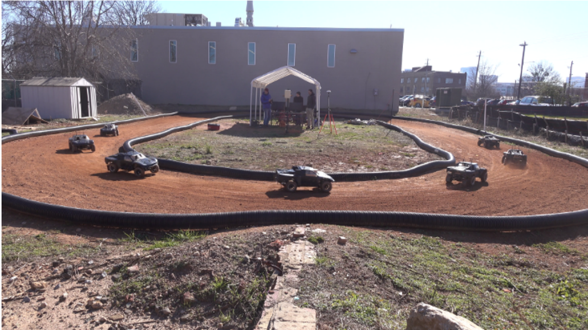
Figure 6.13: Time-lapse image of the vehicle making a cornering maneuver. Notice how the front left wheel is off the ground as the vehicle enters the turn.
