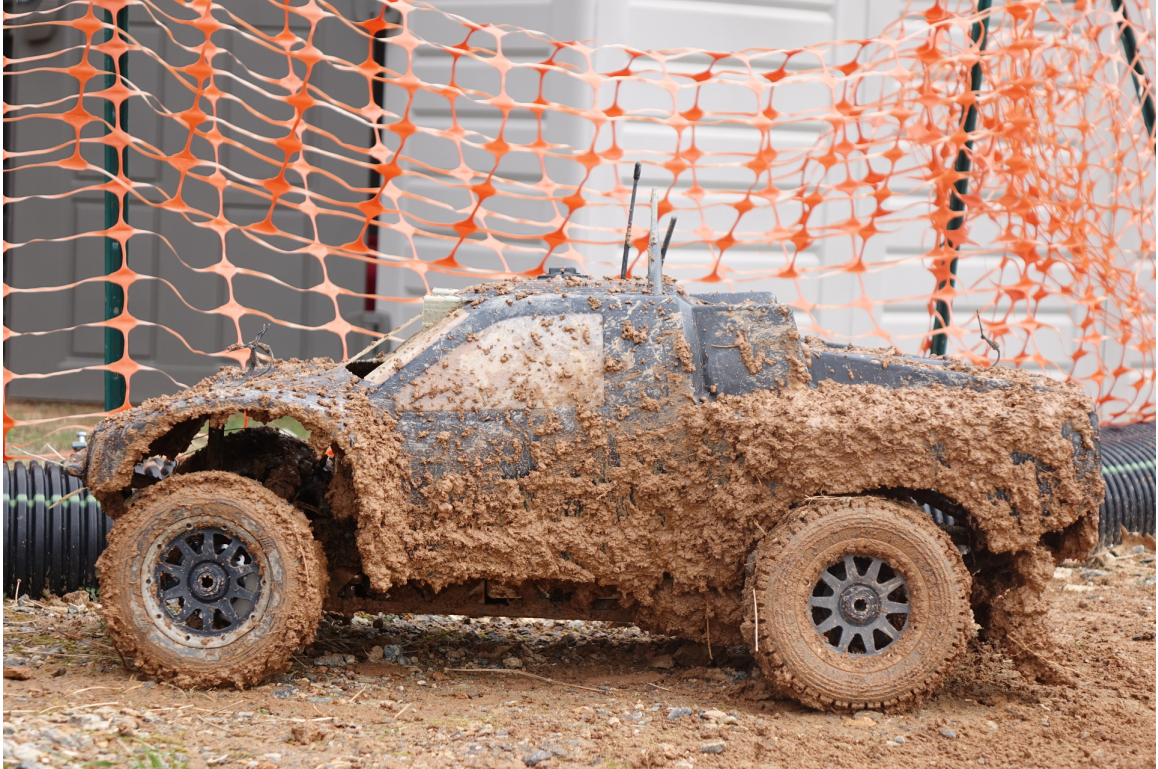
Figure 9.2: AutoRally vehicle after running on muddy surface. Notice the depressed rear suspension, which is caused by the extra weight from the mud accumulating on the chassis and body.
