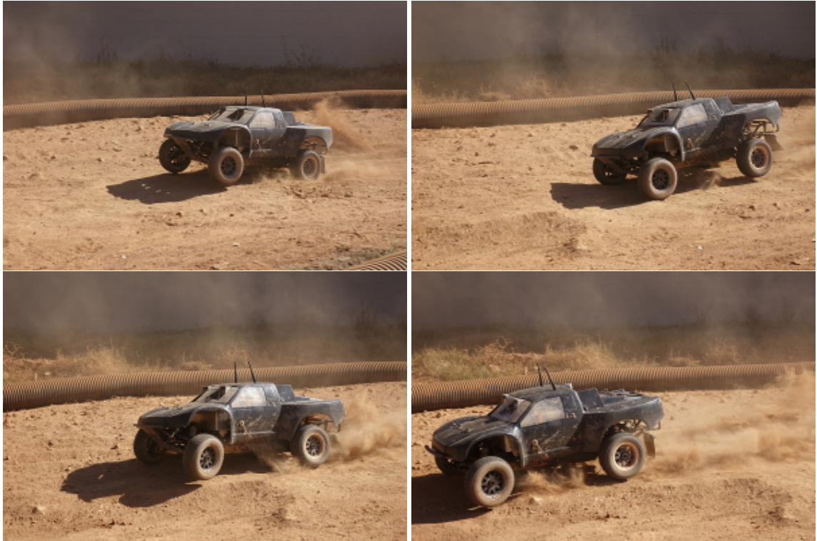
Figure 6.17: Disturbance rejection by the MPPI controller. The car hits a large hole in the track and the front and rear wheels leave the ground in alternating fashion while the vehicle is attempting to steer around the corner.
