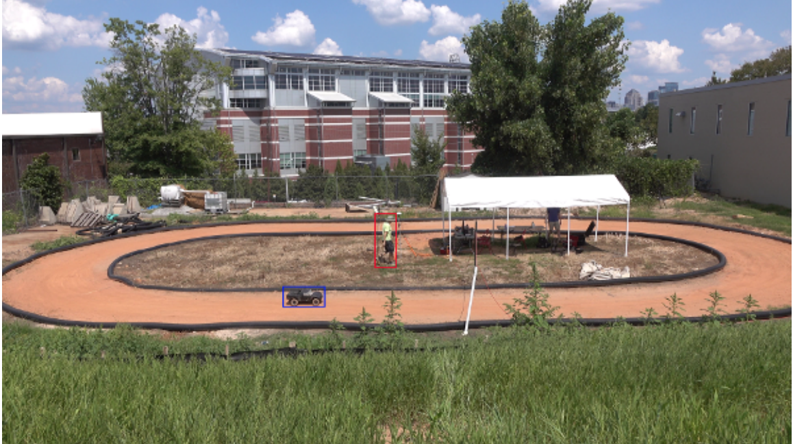
Figure 6.11: Experimental setup at the Georgia Tech Autonomous Racing Facility. All of the state estimation and control software is run on-board the robot itself, making it fully-autonomous and self-contained.
