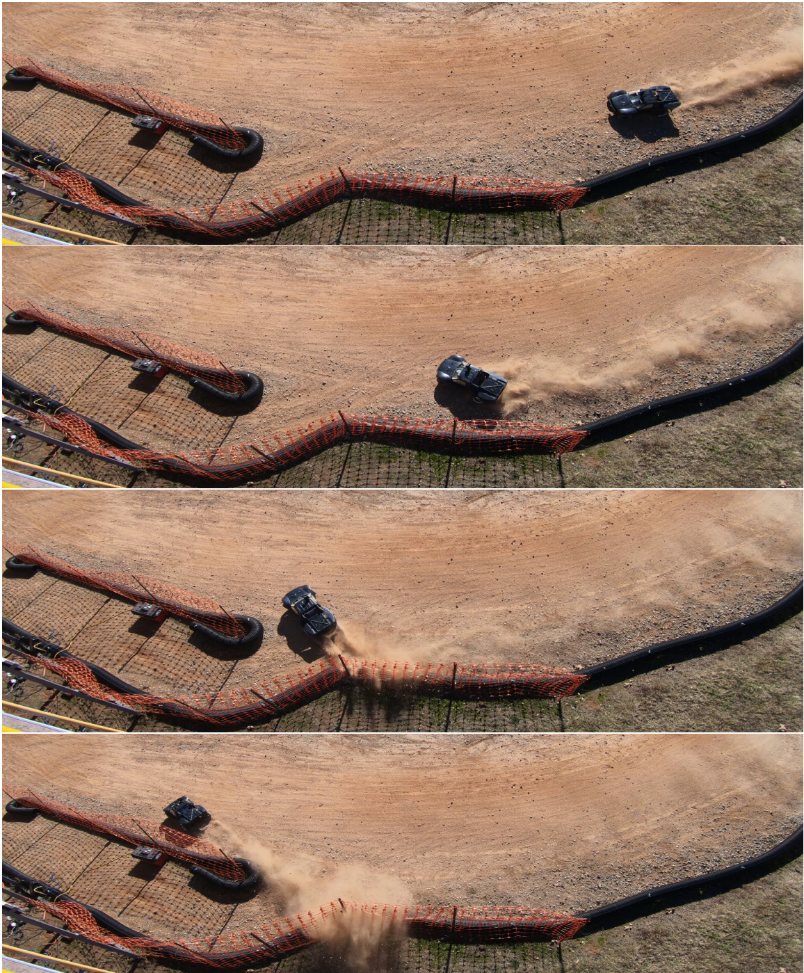
Figure 8.6: Aggressive maneuver by R-MPPI in order to avoid the barrier. Note that the augmented importance sampling is active here.
