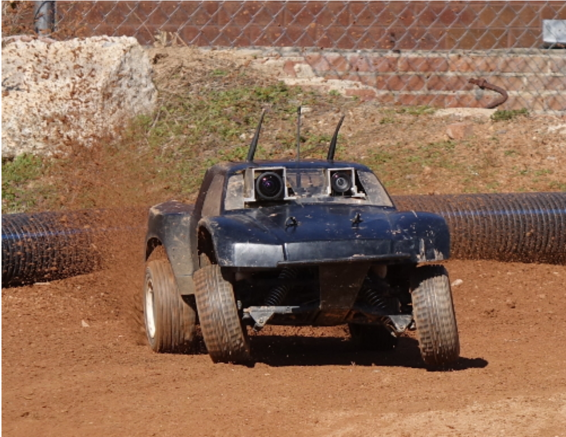
Figure 6.14: Example of the AutoRally executing a controlled powerslide while cornering while under the control of MPPI.
