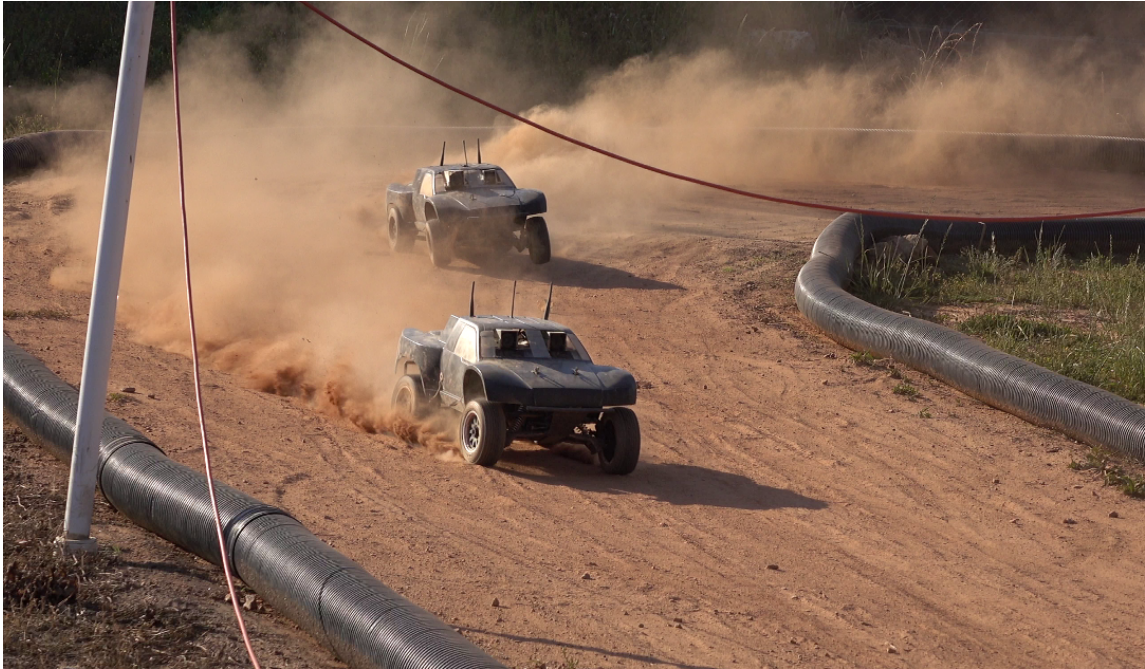
Figure 10.1: Two AutoRally vehicles operating on the dirt test track at the Georgia Tech Autonomous Racing Facility.
