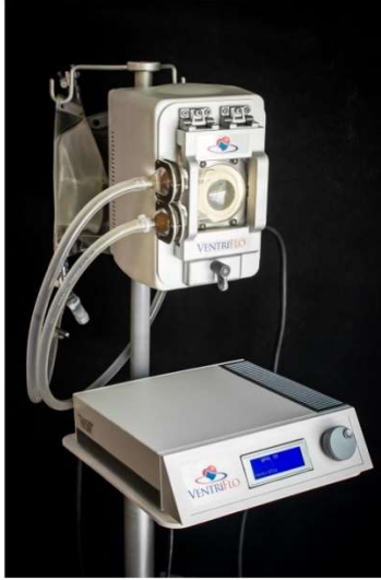
Figure 4-7 VENTRIFLO™ True Pulse Pump.
