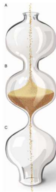
Figure 3-20 Simplistic representation of flow through several constrictions. Only the most severe constriction (c) will determine flow rate.
