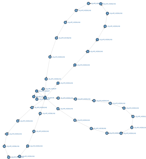
Figure 7.15: Knowledge graph resulting from the modelling of drafted cantilever beams for varying requirements where the loops indicate different requirements.
