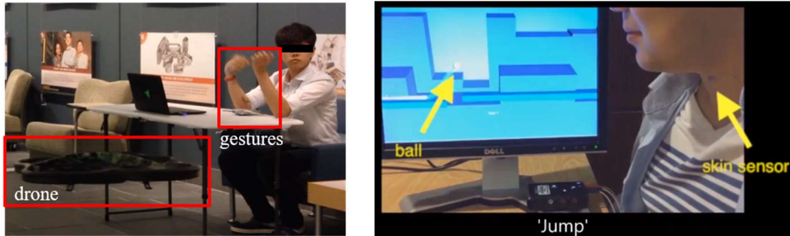
Figure 7. Example of human-machine interface controlling a drone with skin-electronics and human-computer interface controlling a game with skin-electronics on throat muscle.
