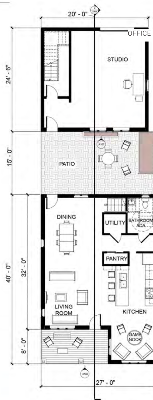
2 FIRST FLOOR PLAN OFFICE OPTION
