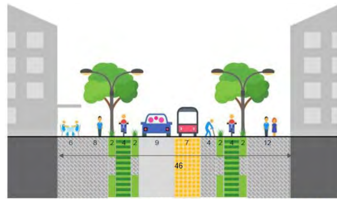
Section of the driven car road - - - -
