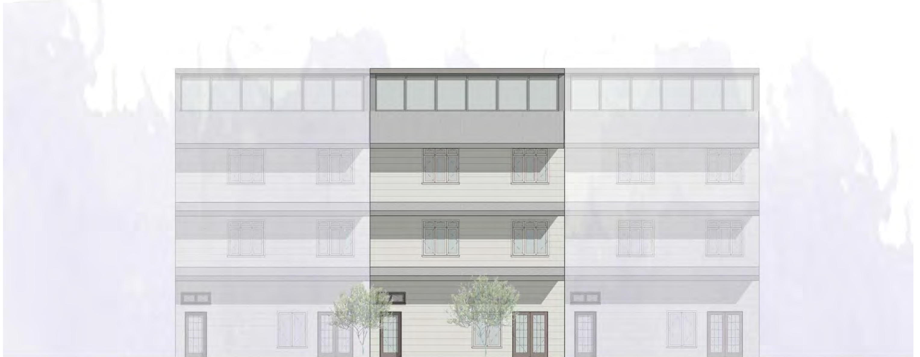
ELEVATION SHOWS THE FRONT OF THE BUILDING WITH THE CLERESTORY WINDOW
