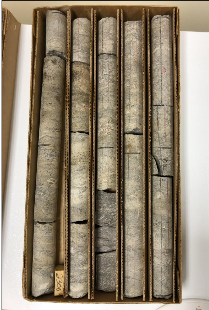
Figure 5. Box 211 from Core 3256, Williams County, Ohio, from top (top right) to bottom (bottom left), box of core covers a depth range of 2290–2300 feet beneath the surface. Each column represents two feet of rock. Core provided by the Ohio Department of Natural Resources.
