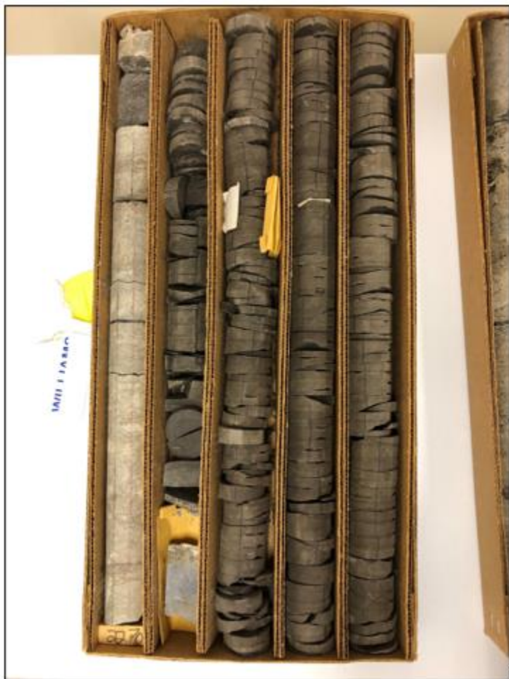
A1: Box 208, Point Pleasant shale from 2260–2267.2 feet and Trenton limestone from 2267.2–2270 feet.
