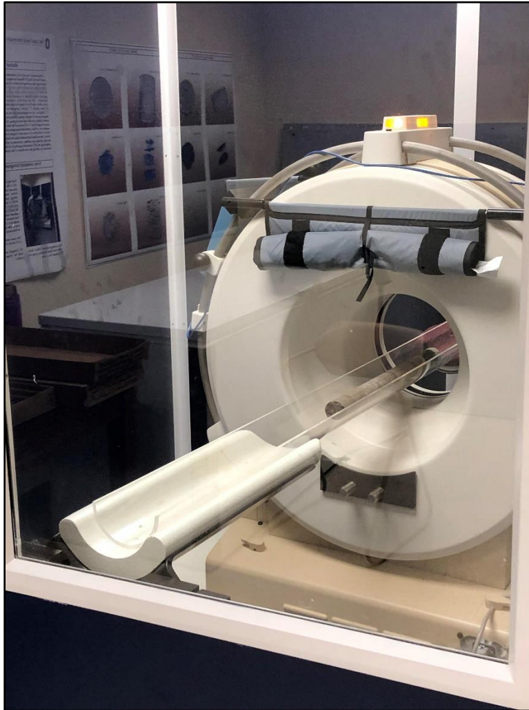
Figure 6. Trenton limestone core being scanned with the XCT scanner in Mendenhall Laboratory, The Ohio State University.
