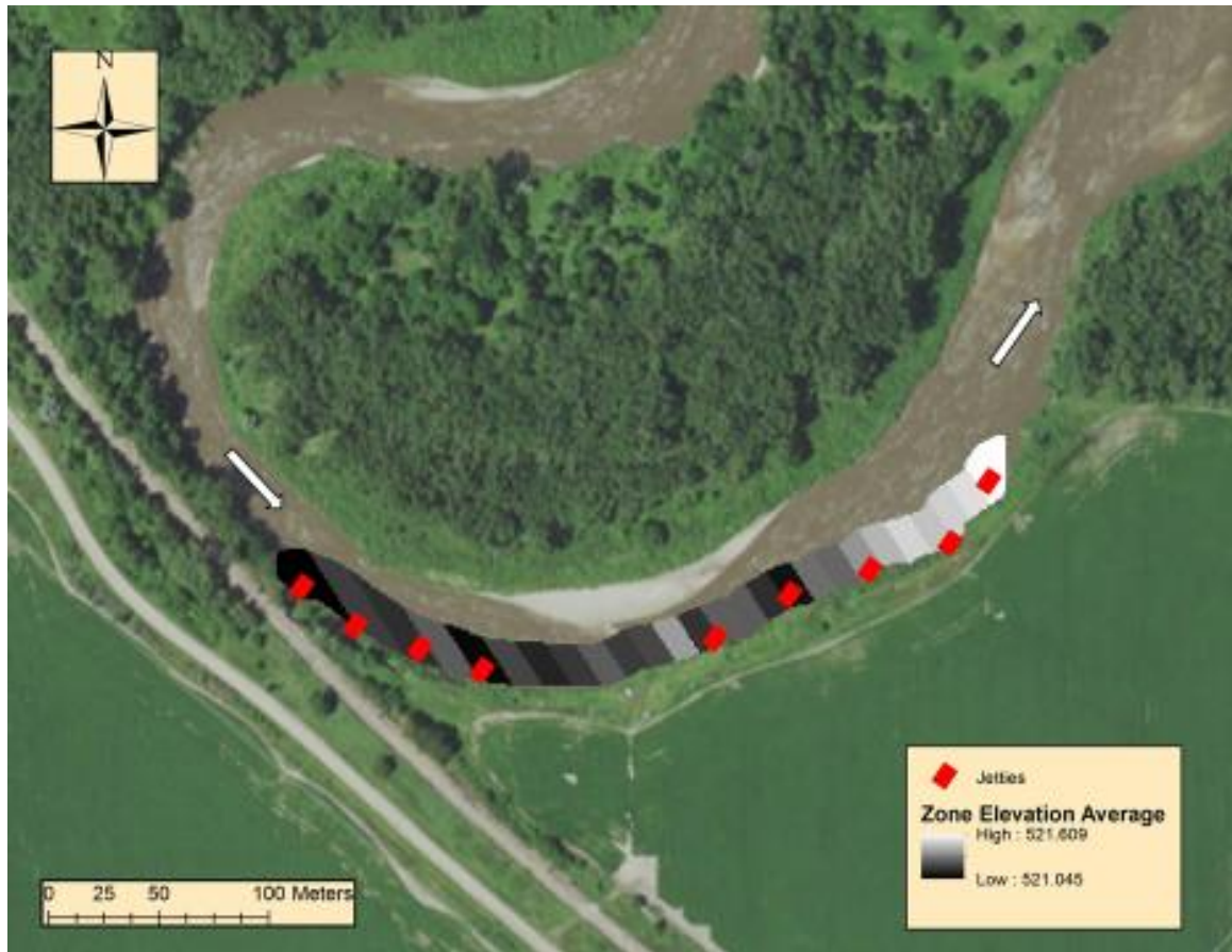
Figure 5. Reach 3 – Zonal analysis of each reach was completed in ArcMap 10.3.1. Each reach was divided into equidistant zones and the average elevation in each zone was used to quantify deposition at the reach.
