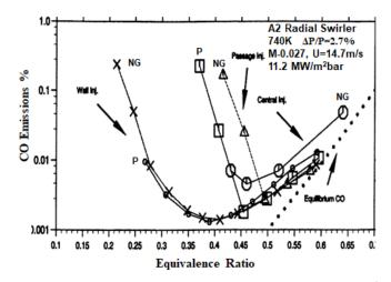
Figure 2 CO Emissions as a function of Equivalence Ratio, Ø.
