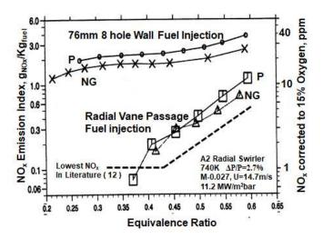
Fig. 7 NO<sub>x</sub> EI g/kg and NO<sub>x</sub> corrected to 15% oxygen as a function of equivalence ratio
