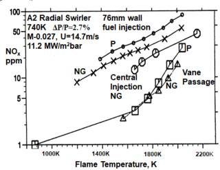
Fig. 6 NO<sub>x</sub> as a function of the adiabatic flame temperature
