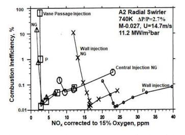
Fig. 8  $NO_x$  corrected to 15% oxygen as a function of the combustion inefficiency.
