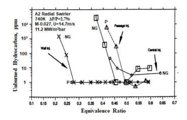
Fig. 3 THC as a function of Ø at 740K
