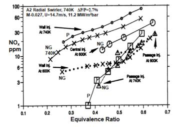
Fig. 5 NO<sub>x</sub> as a function of Ø
