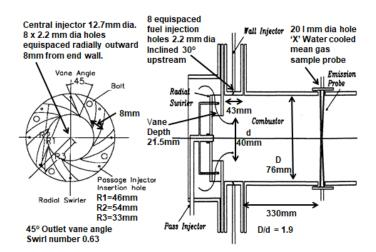
Figure 1 Radial swirler geometrical configuration.
