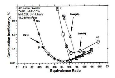
Fig. 4 Combustion Inefficiency as a function of Ø
