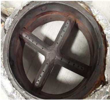
Fig. 10 The 20 holes mean gas sampler
