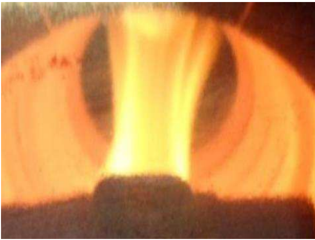
Fig. 9 View of a typical biomass flame through the chamber observation window
