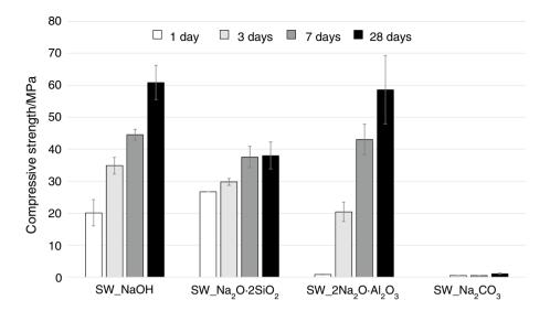
Fig. 2 Unconfined compressive strength of alkali-activated glass wool samples between 1 and 28 days
