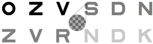
Figure 1. The first test, direct translation of paper PR to ePR. Grayscale was derived from the original PR grayscale. In the inset, a small region of the letter S is magnified to show the chessboard pattern used to compose the appropriate shade of gray.
