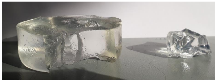
Figure 3-30: Acrylamide gel containing sodium alginate (left) and with added \text{Ca}^{2+} solution (right).
