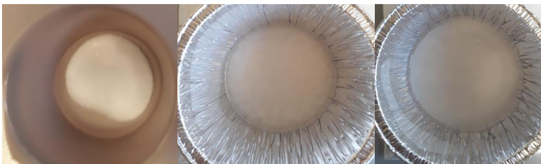
Figure 3-25: standard 3 ml volume hydrogel, 10 wt% p(HEMA) (left), 10 wt% p(HEMA) hydrogel (middle) and 5 wt% p(HEMA) hydrogel (right) all with excess water on top.
