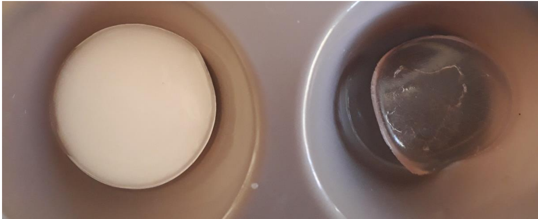
Figure 3-24: P(HEMA) hydrogel as synthesised from aqueous solution (left) and after being dried to the xerogel state (right).
