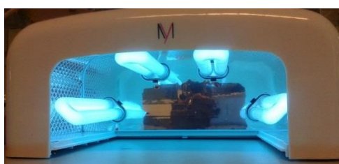
Figure 7-3: UV nail lamp that was used as an alternative UV light source.
