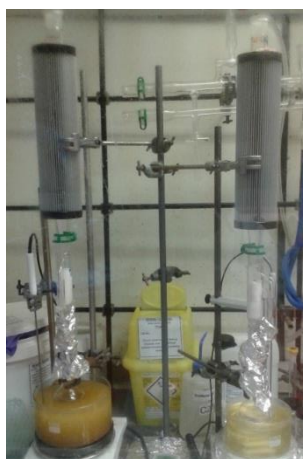
Figure 7-4: Side-by-side Soxhlet extraction set-up.
