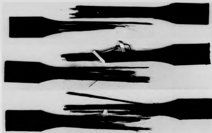
Figure 4.1: Typical failed unidirectional specimens at different strain rates - 5(top), 50(middle) and 500(bottom)[mm/min] crosshead displacement rate.
