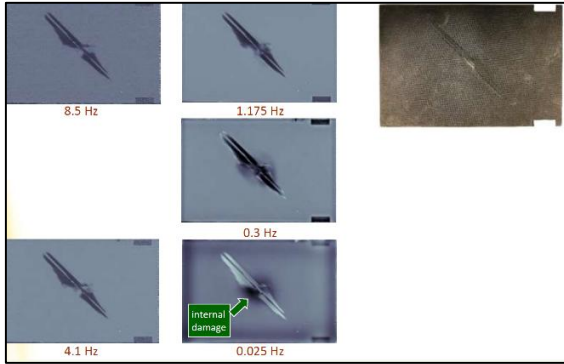
Figure 9: Sample 20 J Demo, Reflection rear face. PPT. The rear face has some substantial damage. The PPT locates the surrounding internal damage [5].
