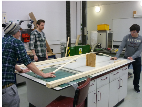
Fig5. The simple testing rig to test the timber battens.
