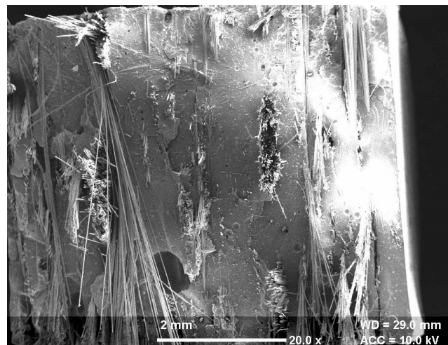
Figure 2. SEM of a cut sectional view of a polymer matrix composite (PMC).
