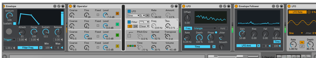
Fig 4.2. Here an array of internal units control the parameters of a software synthesiser to create complex, unconventional timbres. In this particular set-up, envelopes and LFOs are used to create periodic, unusual or rapid changes in the parameters of the ‘operator’ synthesiser, creating unfamiliar timbres and effects that might be difficult to create if one was inputting the parameter data by hand. Creating these sounds may not have a useful output in the moment, but may become useful during future composition.
