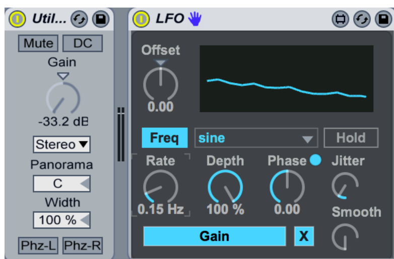
Fig 3.4. The LFO controlling the gain parameter of the utility unit.
