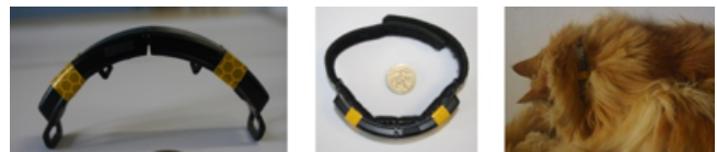
Figure 1. PawTrax. Left: two-part case. Center: collar and case (with 23mm diameter coin). Right: device on cat.
