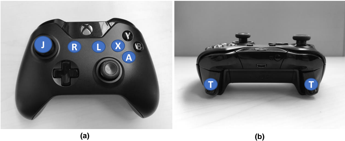
Figure 7. The Xbox controller: (a) shows the top view with the left-hand joystick [J] used to control the 2D movement on the X - Z plane whereas (b) shows the front view with the two triggers [T] responsible for vertical movement along the Y axis. The other action buttons indicated in (a) have the following meanings: [R] for reload of the visualization; [L] for loading next dataset; [A] for selection of an interactive item; and [X] for moving or rotating the scatter plots.
