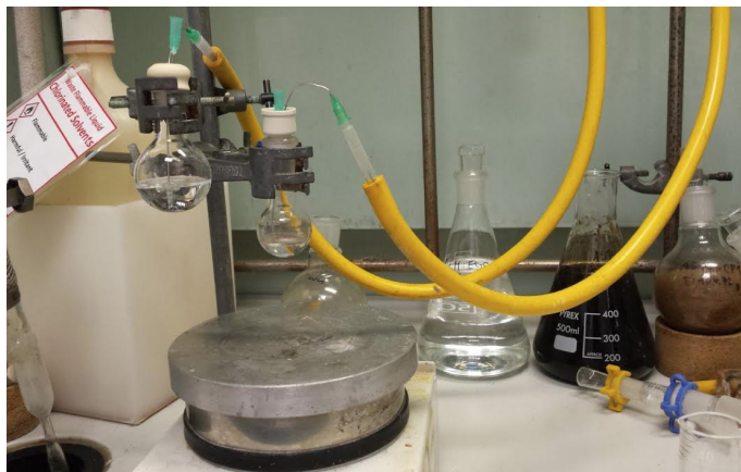
Figure 3.5: ‘Click’ reaction set up in the hood. To ensure no presence of the oxygen the reaction was performed under nitrogen. This protects copper(I) from oxidation which is crucial for the reaction.
