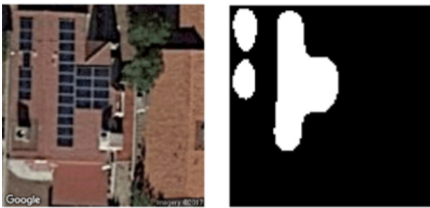
Fig. 6 Automated solar panel location and size estimation through deep learning techniques based on satellite imagery. On the left is the location and size of solar panel as detected by satellite imagery; on the right is the re-constructed image based on deep learning method 110 .
