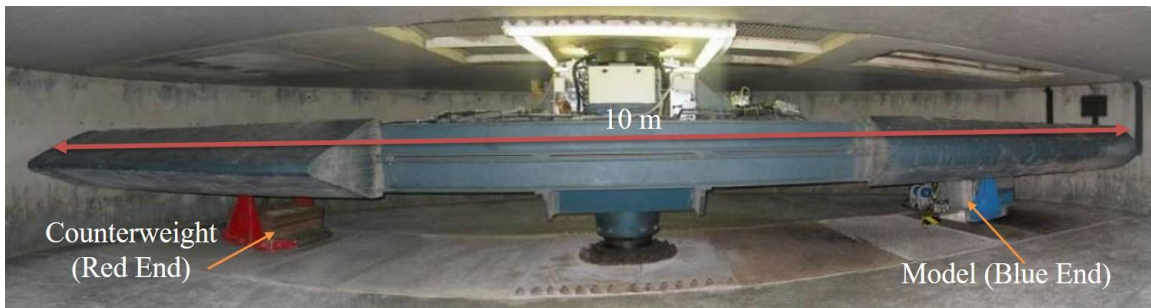
Figure 3.2 - Turner beam centrifuge at Schofield Centre.
