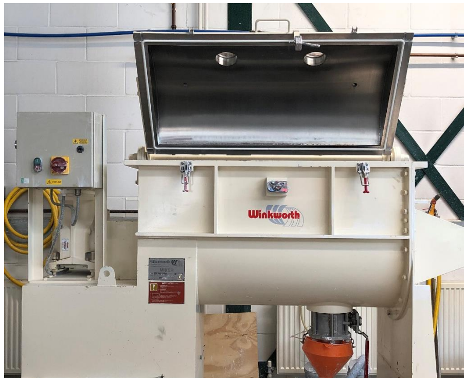
Figure 3.9 - Clay mixer at Schofield Centre, University of Cambridge.
