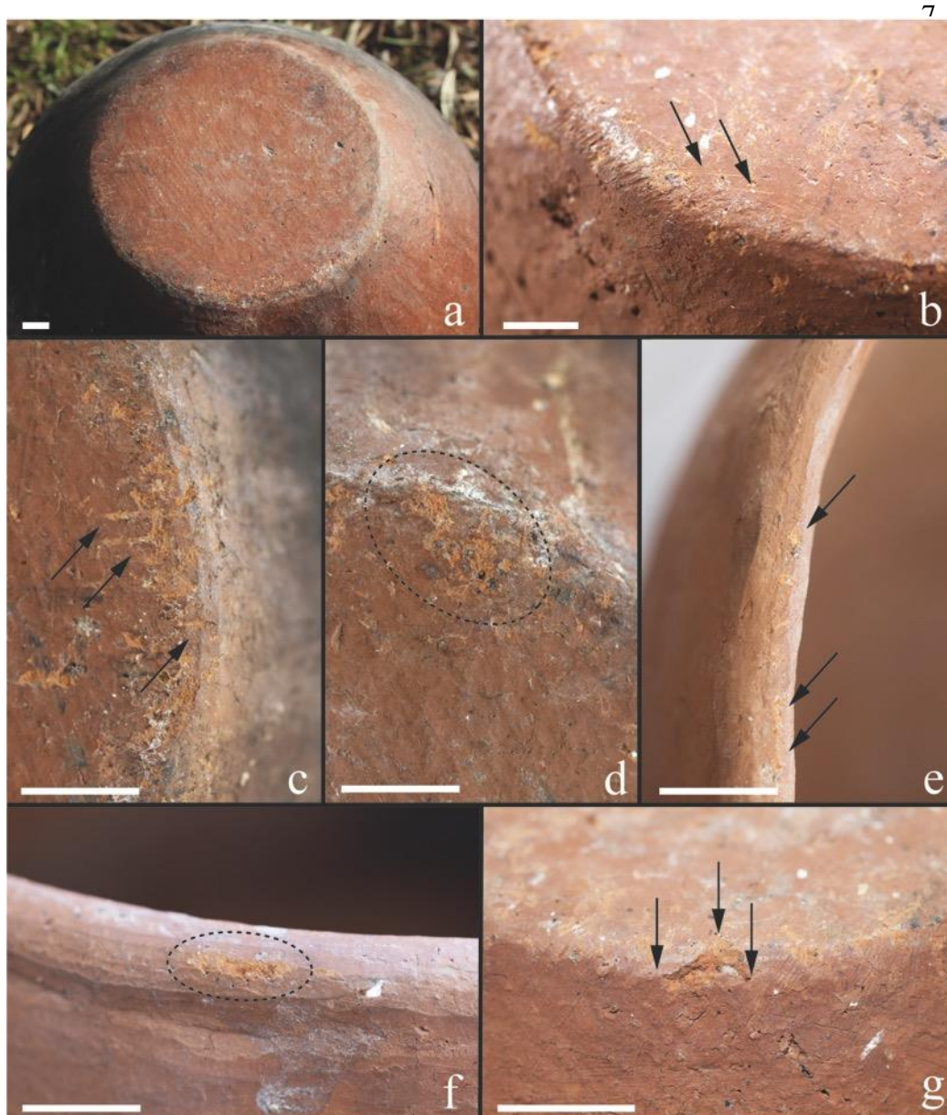
Figure 6 - Abrasive wear and fatigue wear identified on the experimental ceramic vessels n. 3 and n. 4. a) General view of the external base of the vessel featuring abrasive processes (Exp. ID 4); b) Striations and scratches (Exp. ID 3) on a flat topography; c) Grooves on a sinuous topography (Exp. ID 4); d) Depressions on a sinuous topography (Exp. ID 4); e) Depression along limited portions of the vessel rim on a sinuous topography (Exp. ID 4); f) Depression lateral to the vessel rim on an uneven topography (Exp. ID 4); g) Spall detachment caused by mechanical stress on an uneven topography (Exp. ID 3) (white bar equals to 1cm).
