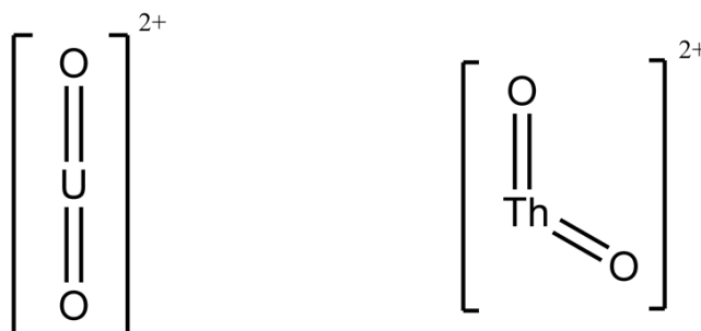
Figure 1.6. A comparison of the linear trans - \text{UO}_2^{2+} species to the bent cis - \text{ThO}_2^{2+} species ( \theta = 122.2 ) 13
