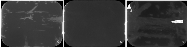
Fig. 1. Blank images of PSP plates with no teeth (Carestream, CS 7600) acquired at the Faculty of Dentistry (University of Toronto).
