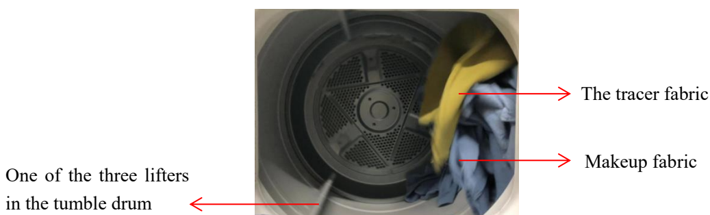
Figure 1 Fabric movement captured in the process of drum rotating in the tumble dryer
