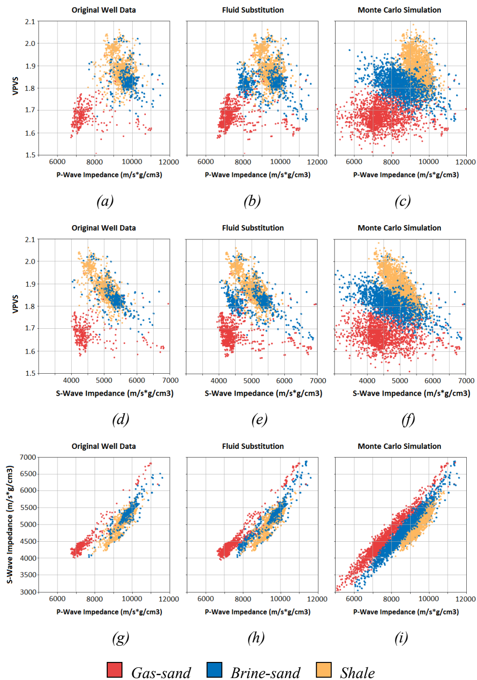
Figure 9: (a)-(c) I_p versus V_p/V_s crossplots in the first row, (d)-(f) I_s versus V_p/V_s crossplots in the second row, and (g)-(i) I_p versus I_s crossplots in the third row. The first column (a, d and g) displays the crossplots using log data from W1. The second column (b, e and h) displays the crossplots using the original well data together with the well data after replacing gas with brine in the sand layers using Gassmann fluid substitution modeling to show the effect of brine on the elastic properties of reservoir layers (A, B and C). The third column (c, f and i) displays the crossplots using Monte Carlo (MC) simulated data using the soft-sand model with intermediate rock physics parameters as shown in Table 1 to simulate a wide range of possible values that might not have been sampled in the well data.
