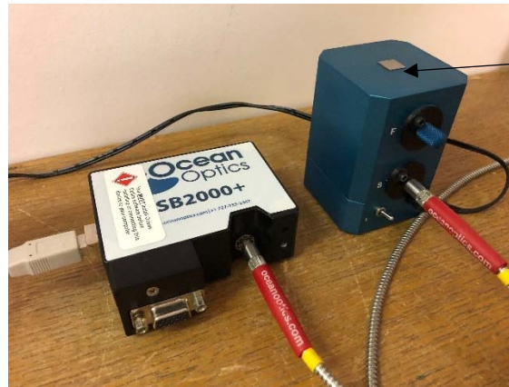
Figure 3 : Optical measurement setup, an Ocean Optics ISP-REF integrating sphere on the right connected to an Ocean Optics USB2000+ spectrometer on the left.
