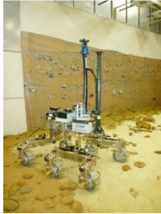
b) Motorised Camera mast on EADS Astrium Mars Rover [7]
