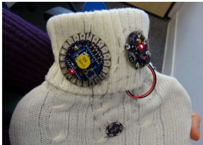
Figure 3.9: Device node - LilyPad circuit including XBee, temperature sensor and power supply sewed onto a study device.
