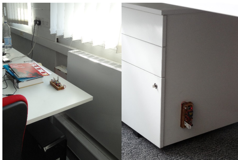
Figure 3.7: Sensor node installation on top of the desk (left) and below at foot height (right).
