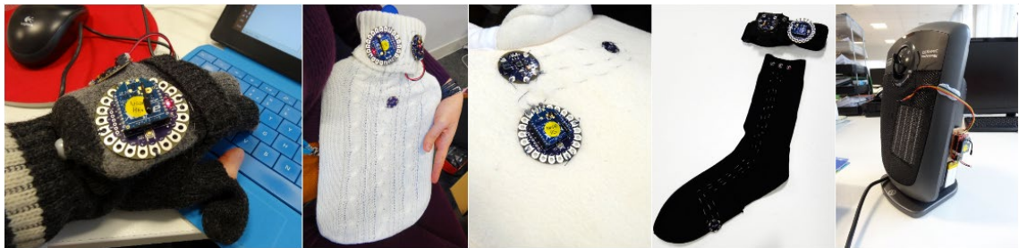
Figure 5.1: Personal Heating Devices used during the study, from left to right: heated gloves, hot water bottle, heated shoulder pad, heated socks, and personal fan heater.
