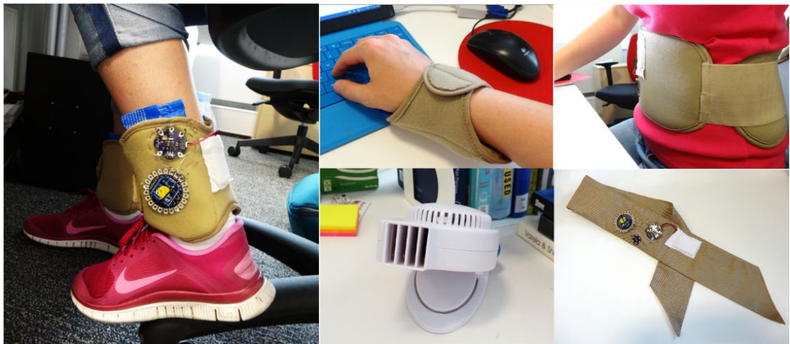
Figure 5.2: Personal Cooling Devices used during the study, clockwise from top left: cooling body wrap, cooling neck tie, wrist cooler, personal cooling fan, and ankle coolers.
