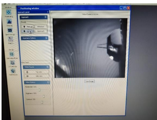
Figure 3-1. Picture showing an example of how close in proximity the probe needs to be to the surface of the mica before approaching.
