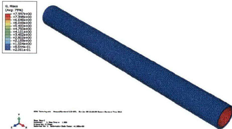
Figure 11. In-vivo arterial layer residual stresses (MPa).
