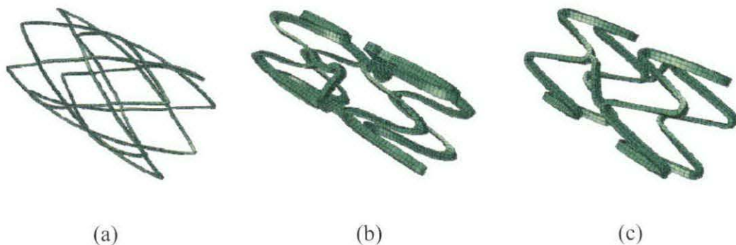
Figure 27. Crimped configurations for (a) stent a, (b) stent b, and (c) stent c.
