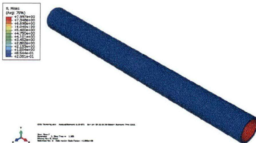
Figure 13. Arterial stresses due to blood pressure (MPa).
