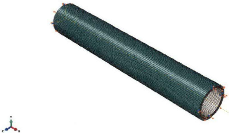
Figure 10. Arterial tethering mesh and boundary conditions.
