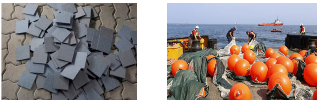
Figure 1 BioBinders and their removal by specially designed net boom. Source: Rostock University
