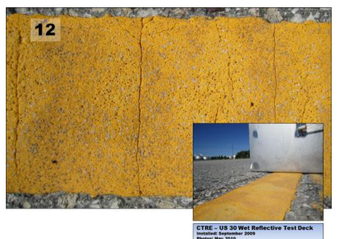
Figure 9. 3M test sections 11 and 12 after one winter
