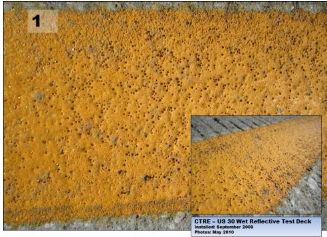
Figure 4. Poly carb test sections 1 and 2 after one winter
