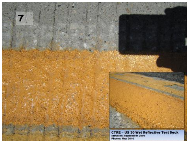
Figure 6. Epoplex test sections 7 and 8 after one winter
