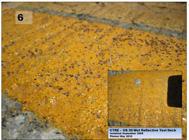
Figure 8. 3M test sections 5 and 6 after one winter
