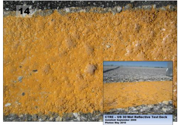
Figure 7. Epoplex test sections 13 and 14 after one winter
