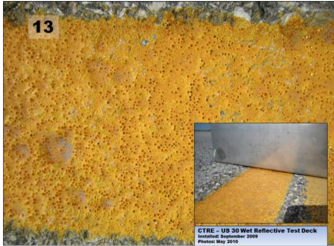
Figure 7. Epoplex test sections 13 and 14 after one winter
