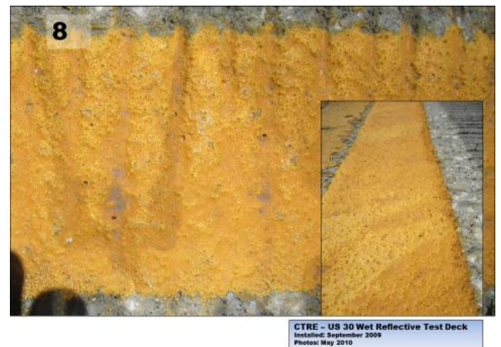
Figure 6. Epoplex test sections 7 and 8 after one winter
