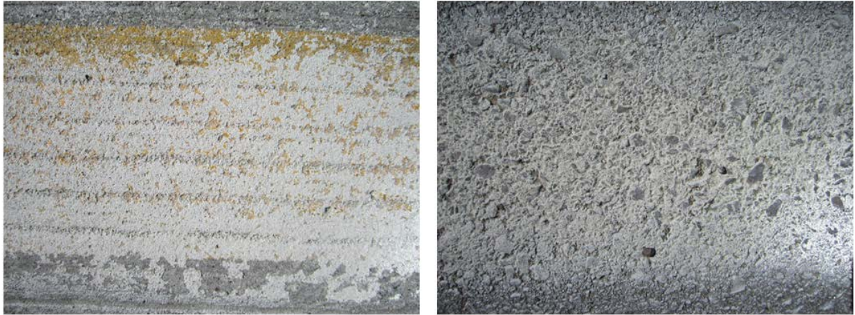
Figure 9. Paint loss (white) after 15 days within the tangent (left) and crossover (right)
