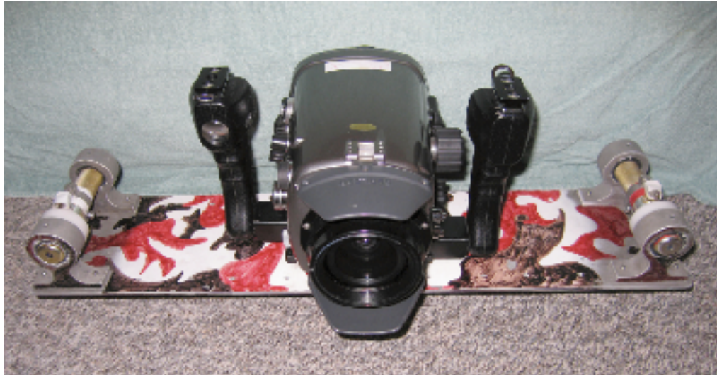
Figure 2. A pair of green, underwater laser pointers mounted in parallel to an underwater video housing.
