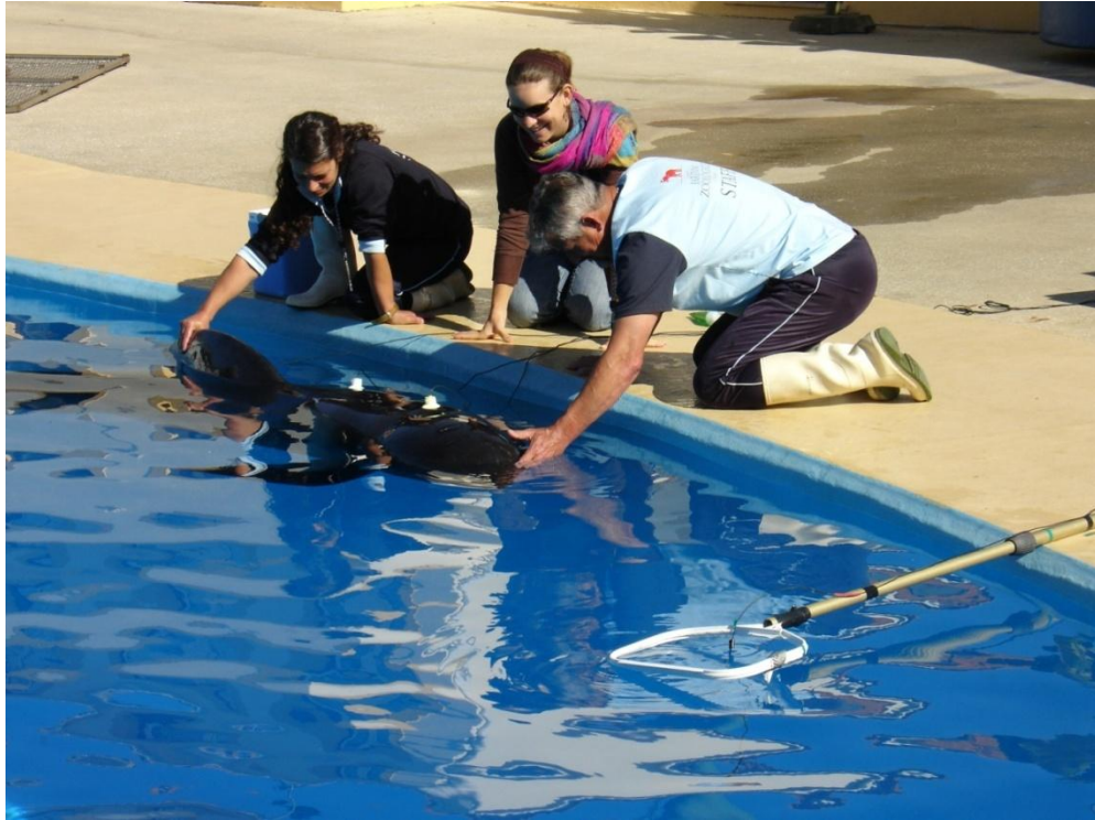
Figure 5: Experimental set-up with the animal wearing electrodes embedded in latex suction cups. The subject remained at the surface one meter away from the hydrophone placed 30cm below the surface.
