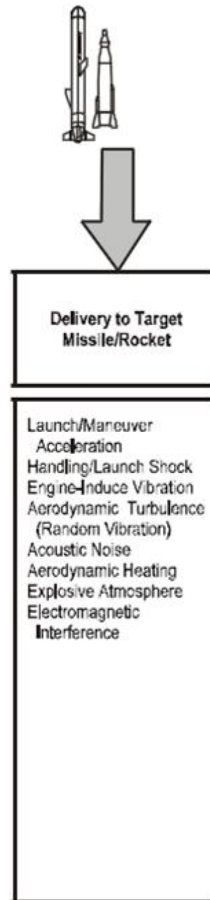
Figure 5.1: Missile Launch Induced Environment from MIL-STD-810G
