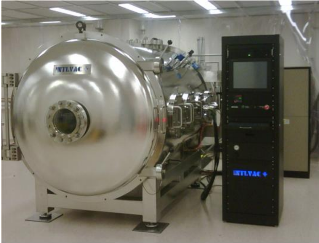
Figure 6.5: HSFL Thermal Vacuum Chamber for Microsatellite Testing
