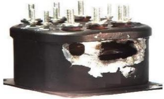
Figure 9.4: Damage to a relay caused by a tin whisker and secondary metal vapor arc, Courtesy of NASA
