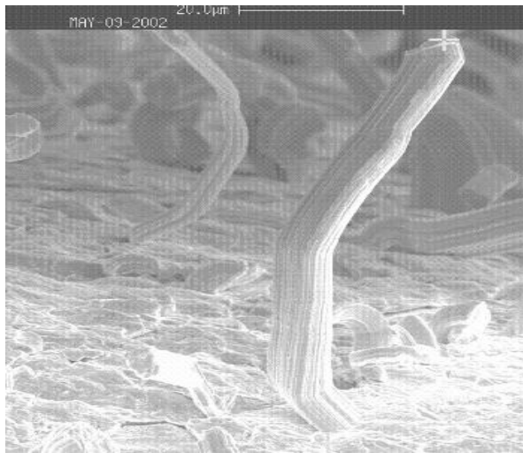
Figure 9.1: Tin whiskers, Courtesy of NASA
