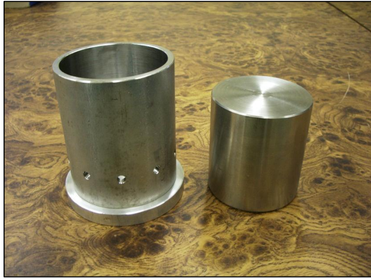
Figure C.3. Fabricated piston for Napier grass fractionation via hydraulic press
