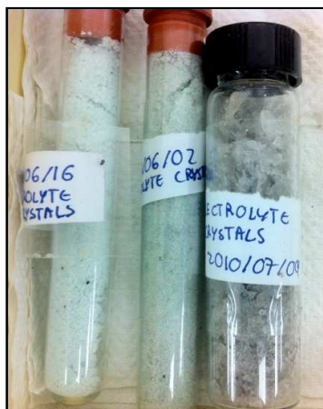
Figure 5.1 Picture of crystal precipitates from the carbon fuel cell showing the presence of nickel carbonate by the greenish tint in the crystals
