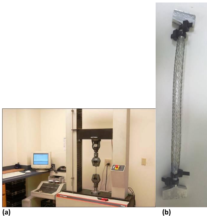
Fig. 3.3 (a): Instron tensile tester (Google Images); (b) Stent mounted onto graspable adapter
