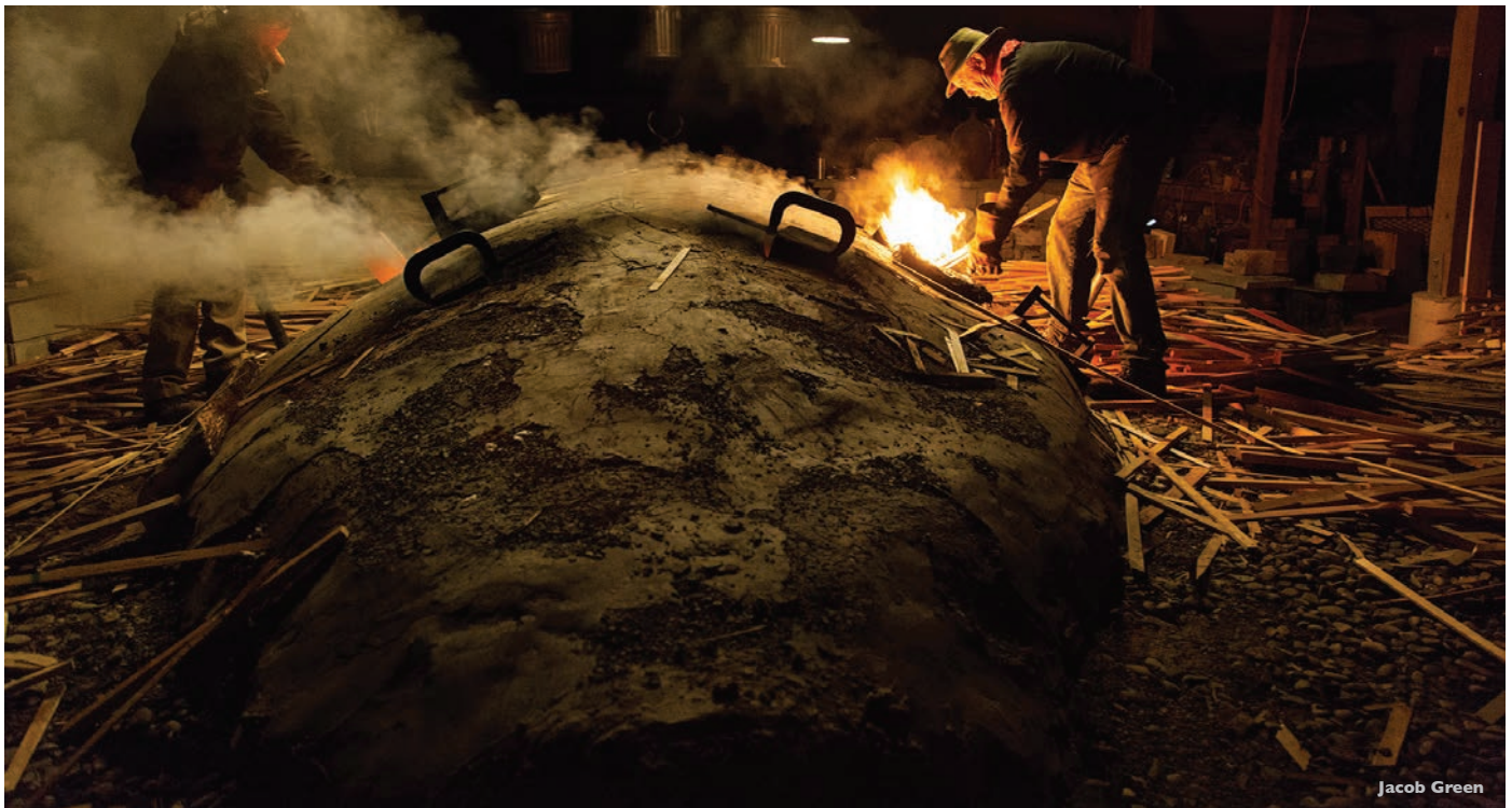
A volunteer feeds a wood-fire kiln at The Clay Studio of Missoula. Missoula is home to one of the largest wood-fire kilns in America, and because of its size, it must be constantly stoked during the seven- to nine-day firing. The kiln is only used a few times per year due to this time commitment.
